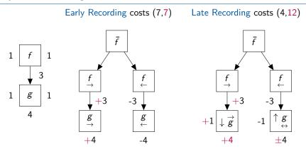
Color coding accesses to memory (black) and contributions to *COST*; mixed colors mark contributions to both, e.g, +4 marks increase in memory requirement by four units (write access). Missing labels are equal to zero. Note: COST = OPS+ write accesses to memory -|V|.
