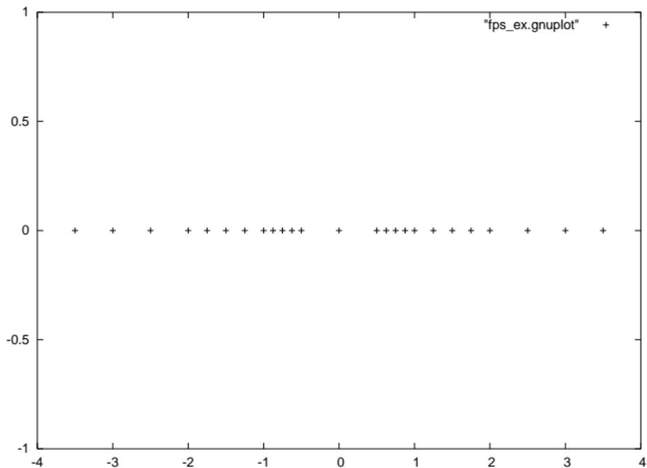
Real values which cannot be represented exactly within the given floating-point number system are typically **rounded to the nearest** representable number.
