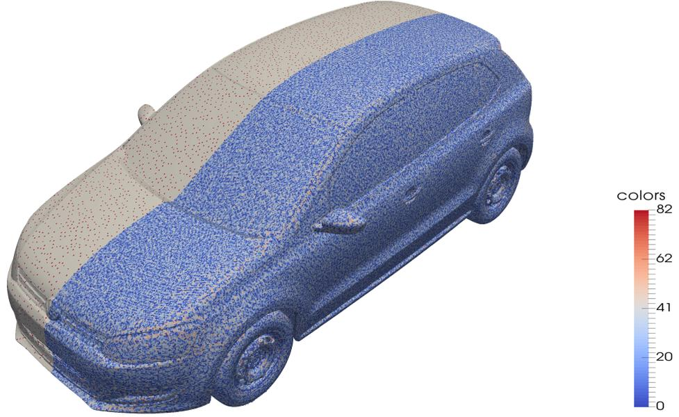
**Figure 4.40:** Cell colors of distance-4 coloring of near wall cells. Plot is split at the  $y = 0$  plane. On the  $y > 0$  half of the plot only cells of color zero are shown in red.
