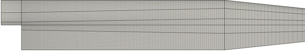
**Figure 5.1:** Geometry of the Pitz-Daily 3D test case with blocks (bold black lines) and cells (gray lines) for refinement level one. Inflow on the upper left, outflow on the right. The geometry is extruded 0.25 m in z-direction.
