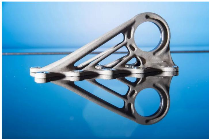
**Figure 1.2:** Structural part of an Airbus A350, optimized for weight. Part sintered from metal by additive manufacturing. Source: Airbus [Air18].
